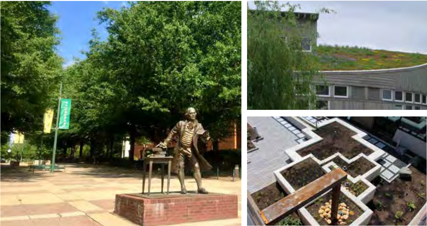
The Civic Campus Typology is characterized by impervious surfaces (L). Green roofs (Top R) and stormwater planters (Bottom R) can mimic the ecological functions of water absorption and filtration that have been lost.
