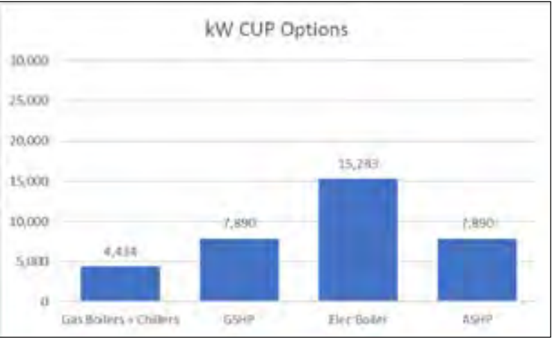
Figure 15: Central Utility Plant Option Electricity Loads (No Gas Boilers)
