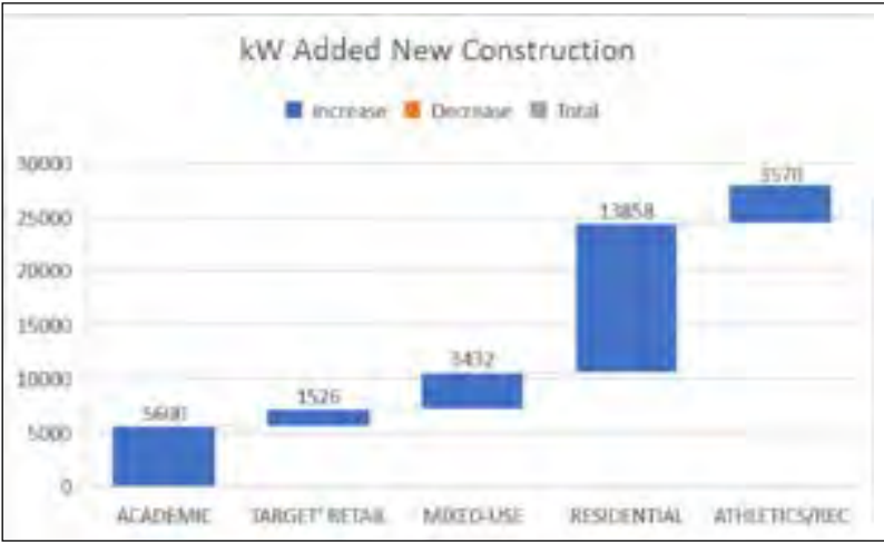
Figure 16: Program Electricity Needs if Domestic Water Heating Occurs at the Building
