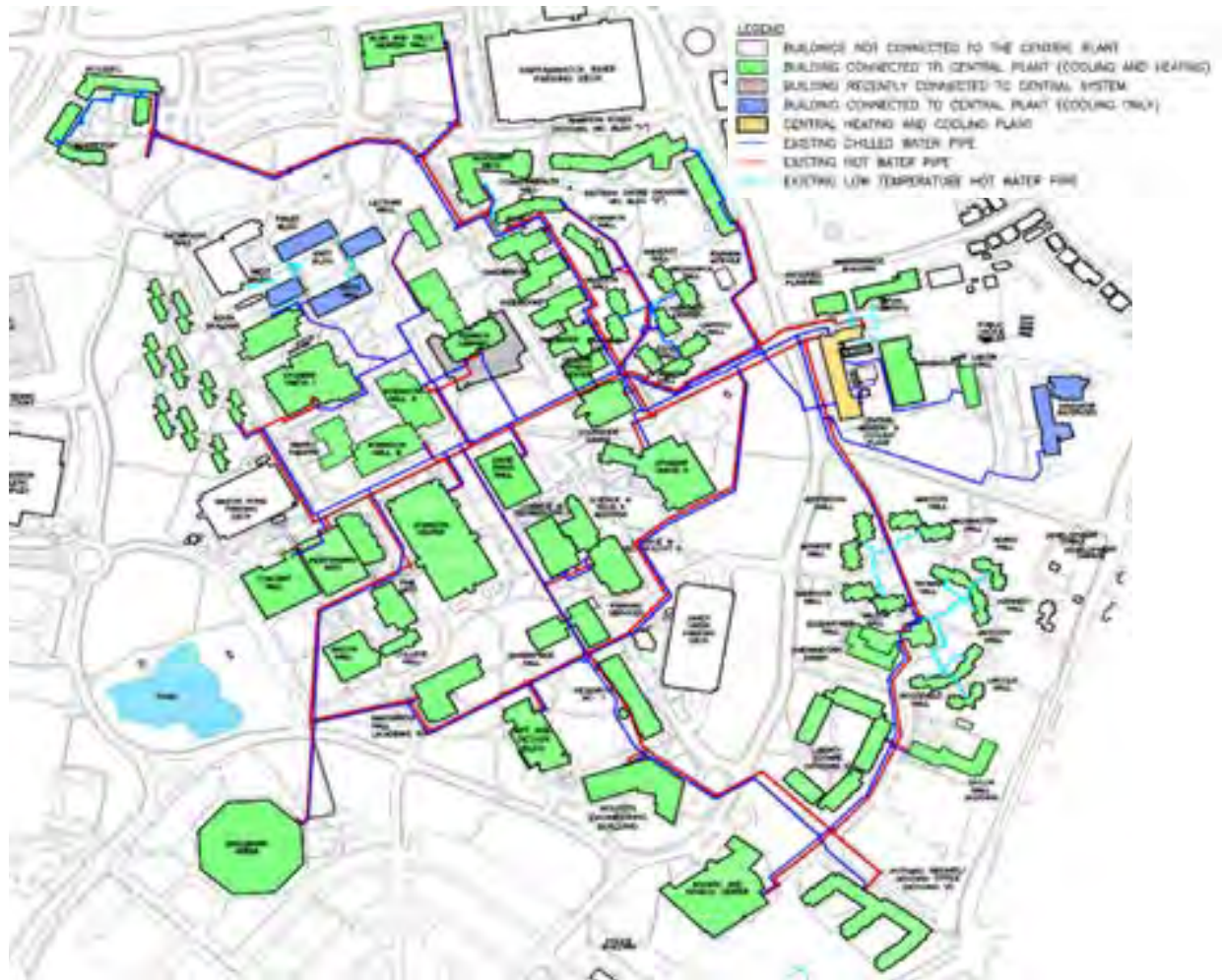
Figure 3 - Existing Central Plant and Distribution Network
