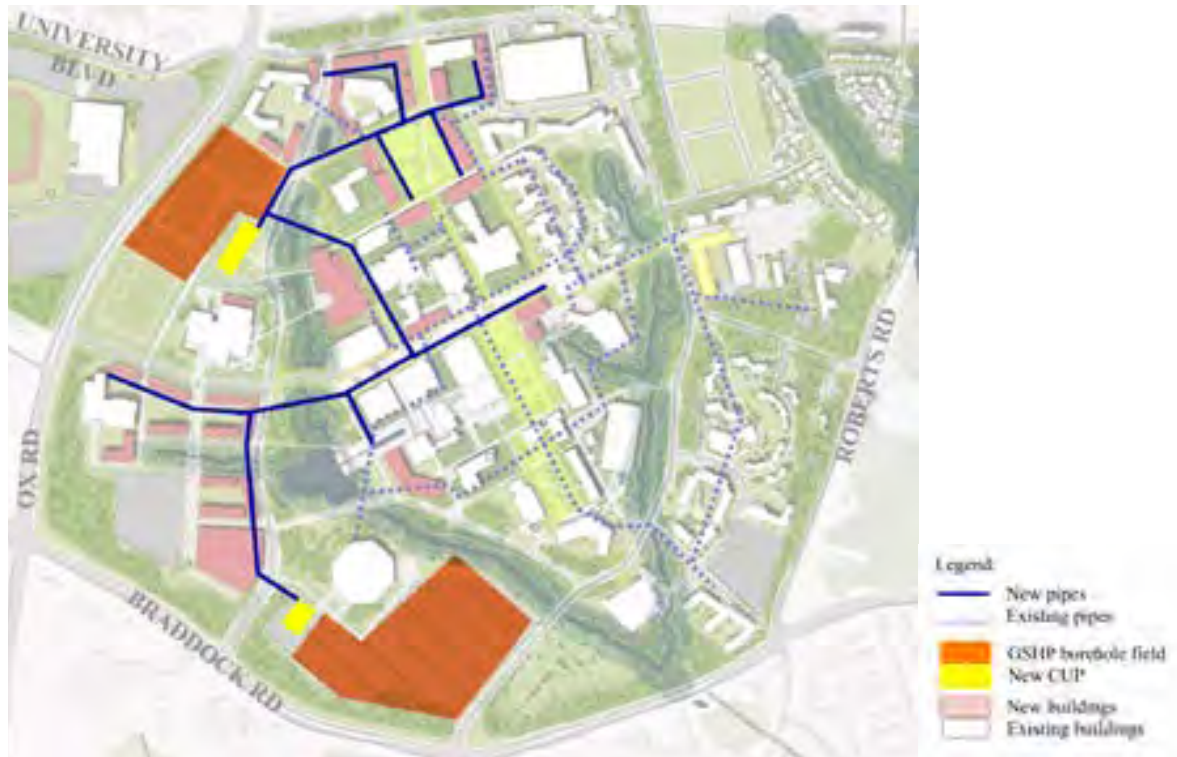
Figure 9 – Option 2 Layout (Central Ground Source Heat Pumps)
