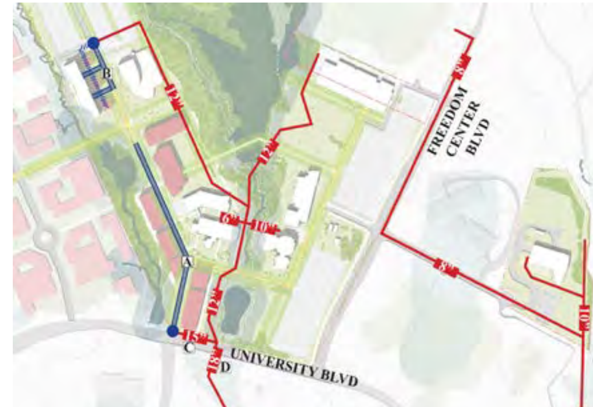
Figure 23 - Proposed Sanitary Sewer Improvements at SciTech Campus
