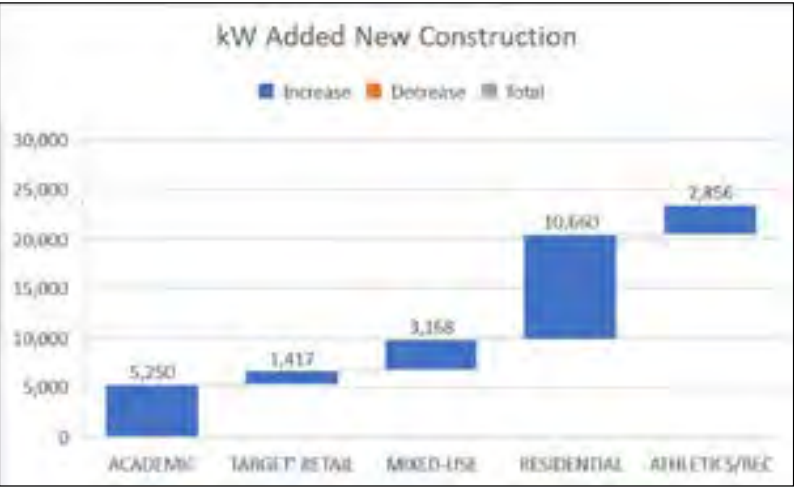
Figure 14: Program Electricity Needs if Domestic Water Heating Occurs at the Central Utility Plant.
